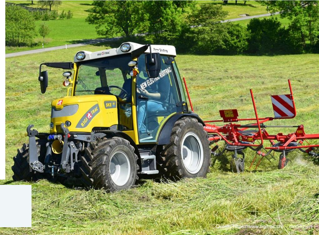
Rigitrac battery electric tractor (Switzerland)
