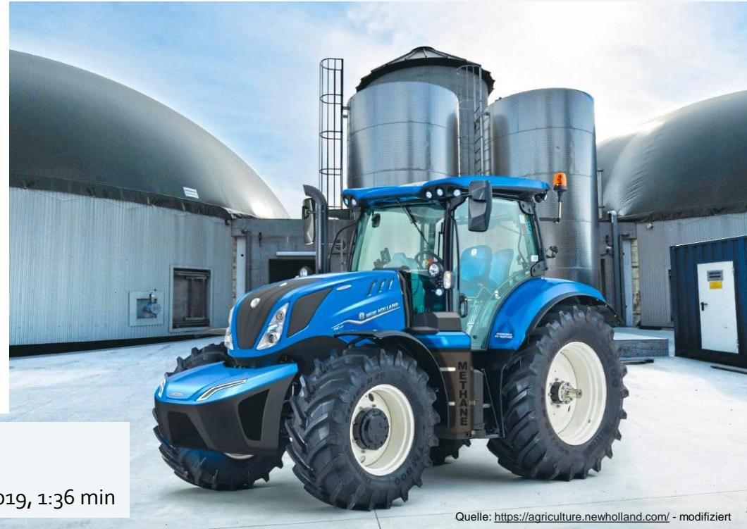
New Holland methane powered tractor
